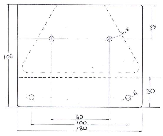
Plate must be galvanised after fabrication, before assembly to ensure the galvanising is not damaged during bending
